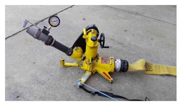
The supply engine was set up on a hydrant using the front intake and a 50 foot section of 3" into the side intake. The engine supplied the portable deck pipe through 50 feet of 4" LDH.
