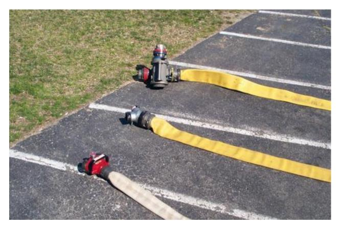
For fire companies operating with 3 inch supply lines a standard 2 ½ inch clapper valve siamese is adequate. For fire companies that operate with LDH, a large clapper valve siamese provides an optimum solution without restricting the available flow to the attack engine.
