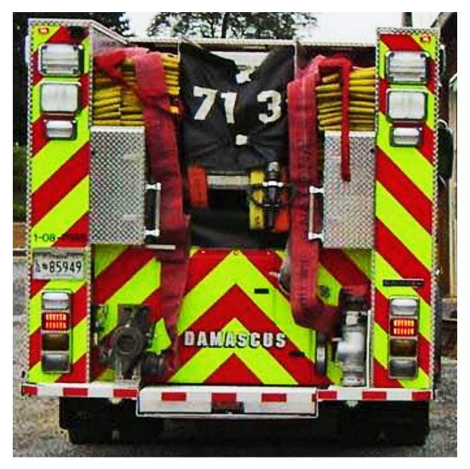
For fire companies that do not operate with split supply line hose beds, the frequency of operations may dictate which device to carry. If the first due is mostly rural, then a siamese would be the appropriate choice. If the area is predominately hydrants, then a hydrant valve would be the appropriate choice.
